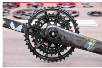
▲The R7 carbon fiber cranks feature one-piece molding technology and weigh 590g.
