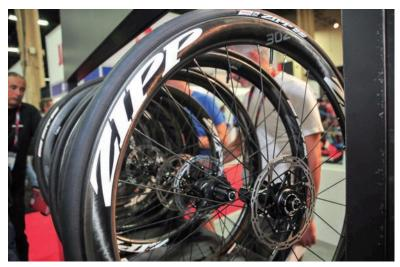
$\blacktriangle$  All of Zipp's NSW wheels reflect disc brake specifications, and also have an all-new rims design and compatibility with tubeless tire systems.
