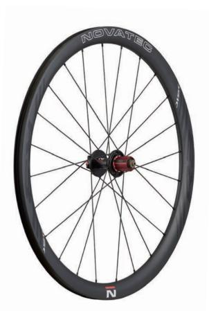
$\blacktriangle$ The Novatec R3 Clincher disc brake uses asymmetric eccentric wheels to ensure that tension in the spokes due to the disc brakes is even on the right and left; the wheels also have greater rigidity, and weigh only 1,630g.
