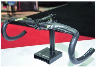
$\blacktriangle$  Zoom Aero carbon fiber handlebars employ a hidden cable routing design to effectively reduce wind resistance.
